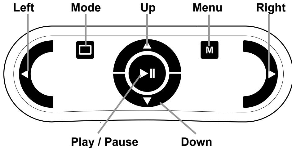
**Play / Pause button:** Round button in the centre of the remote control to stop and restart reading. Press and hold down the button for 2 seconds to spell the current word. Pressing the Play / Pause button within the menu will activate the button, cycle through the available options, check or uncheck the selection or enter a submenu.
