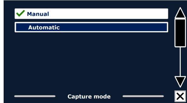
Automatic mode is recommended when capturing multi-page documents for a more streamlined reading experience. It also works well for single-page captures, especially if you capture numerous single-page documents. The motion detector can respond to unintentional movement, such as a desk being shaken or a hand passing under the camera; therefore, reduce the amount of time between scans to minimize the risk of an accidental capture.
