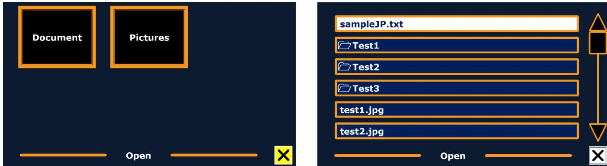
Scroll through the list of documents or pictures using the Back button or Forward button on the ClearReader<sup>+</sup>, or the arrow keys on the Magnification Feature Pack. Open a document by pressing the Play / Pause button.
